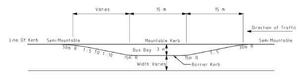
Diagram 1 \_ A typical bus-stop layout – Austroads Guide to Road Design –Geometric design Fig 4.39, dimensions are the critical feature, no requirement for kerbing etc,
