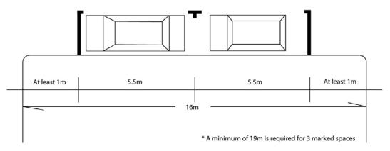
*Diagram 1\_Parking Bays need to meet the Australian Standard. There is room for 2 bays of 5.5m by 2.6m*
