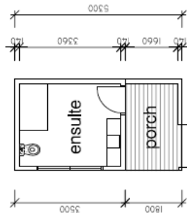
Floor Plan 1:100 GROSS FLOOR AREA - 10.2M 2 GROSS PORCH AREA - 5M 2
