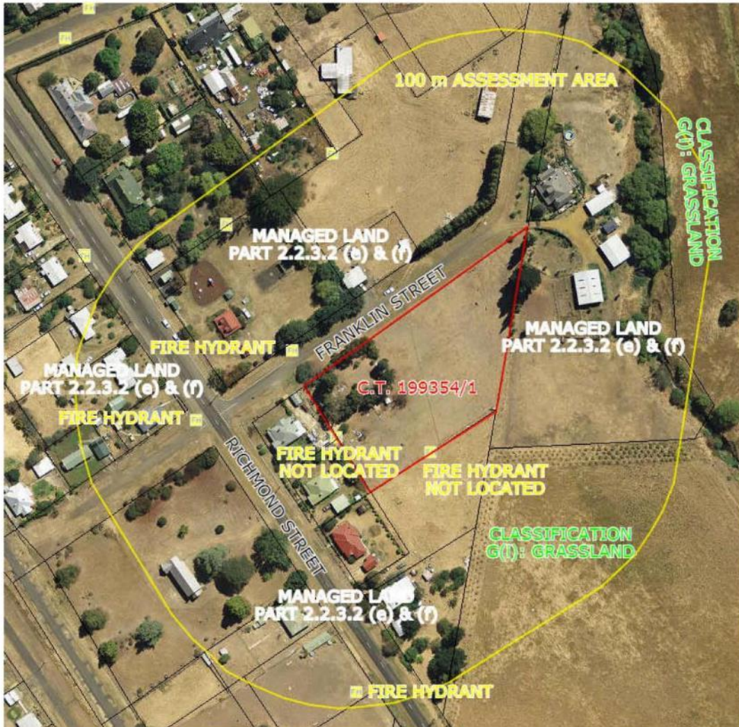
Image 8: Predominant vegetation surrounding the site Note: fire hydrants not located are as shown in ListMAP and are assumed to be erroneously mapped
