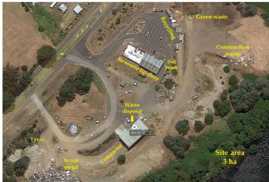
Figure 12: Layout of Huon Valley Council's Southbridge waste transfer station
