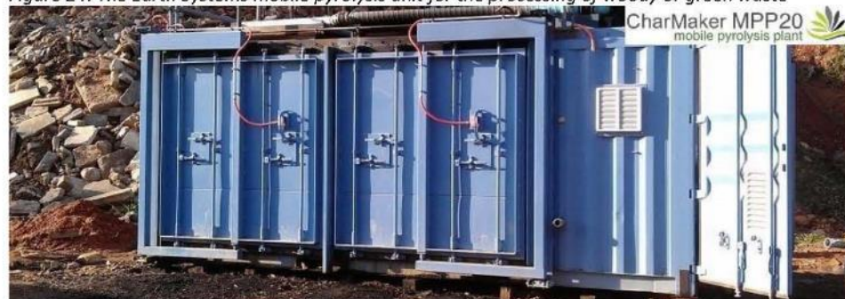
Figure 24: The Earth Systems mobile pyrolysis unit for the processing of woody or green waste
