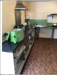
Kiosk / kitchen will require a substantial upgrade to be compliant. Minimum requirements are a double bowl sink, hand washing sink, splashbacks and coved vinyl floor.
