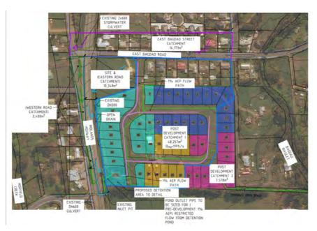
Image 8 - Proposed Stormwater Catchments
