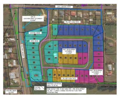
Image 3 - Proposed Stormwater Catchments
