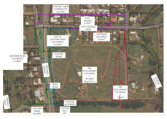
Image 2 - Existing Stormwater Catchments
