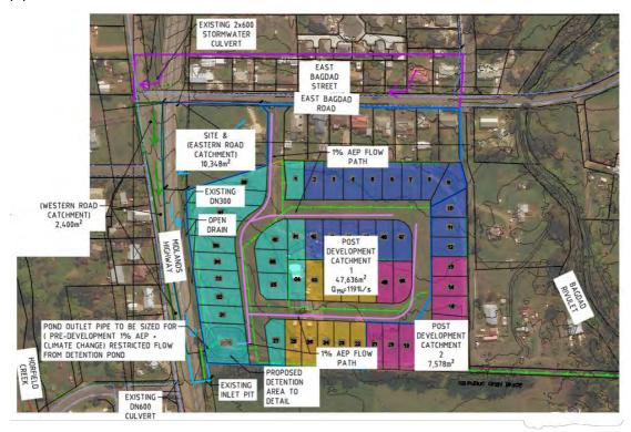
Image 5 - 1% AEP + C.C. Overland Flow Path
