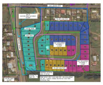
Image 3 - Proposed Stormwater Catchments
