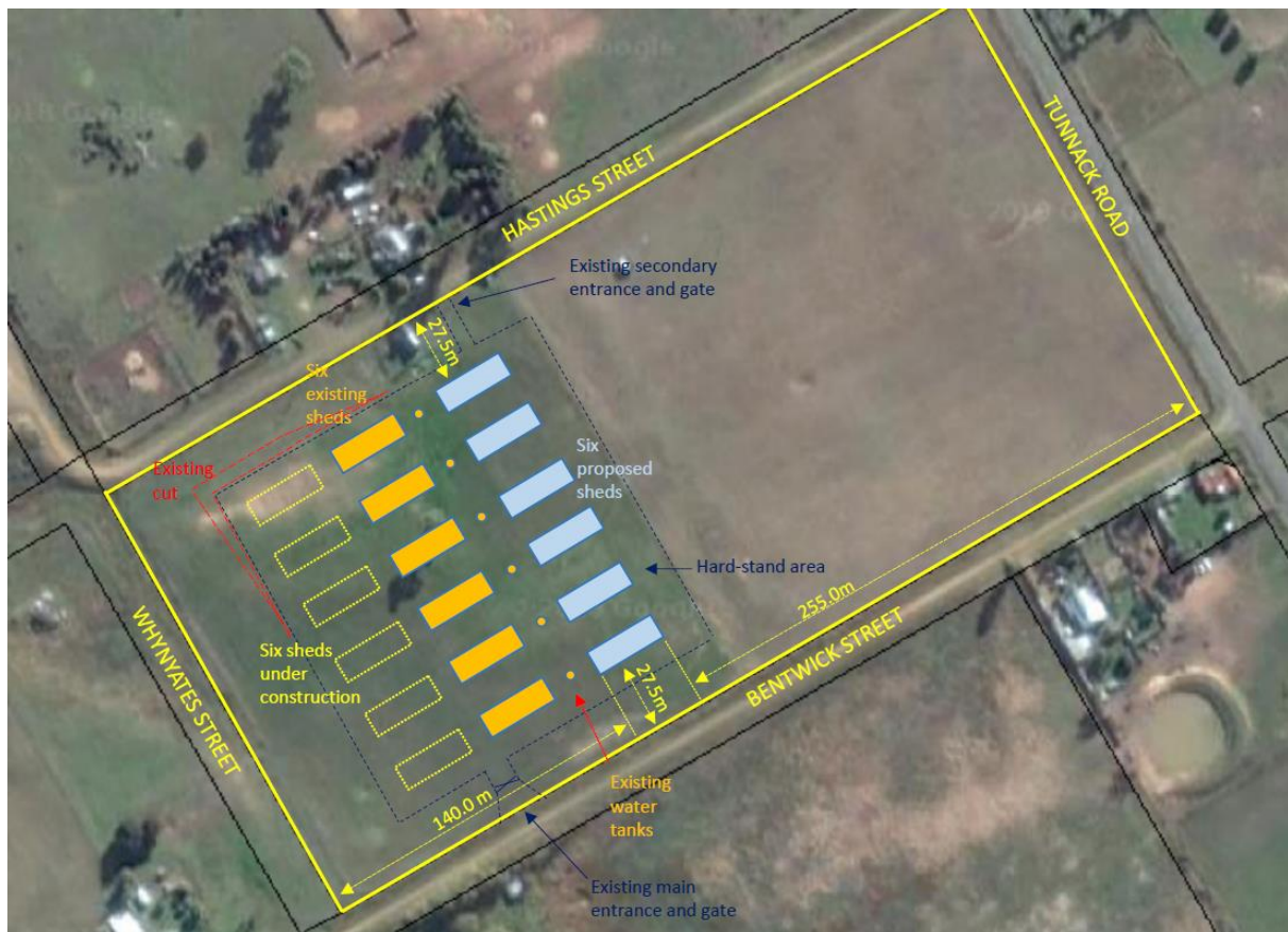
Figure 1: Site plan with existing sheds shown in orange, sheds under construction shown with yellow dashed outline and proposed sheds for bushfire assessment purposes shown in blue.
