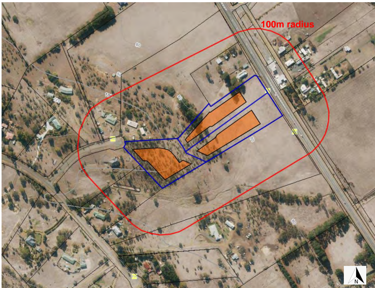
Figure 1: contoured listmap. www.thelist.tas.gov.au Subject property and proposed lot structure outlined in blue with proposed building areas in orange. Fire hydrants are yellow squares.
