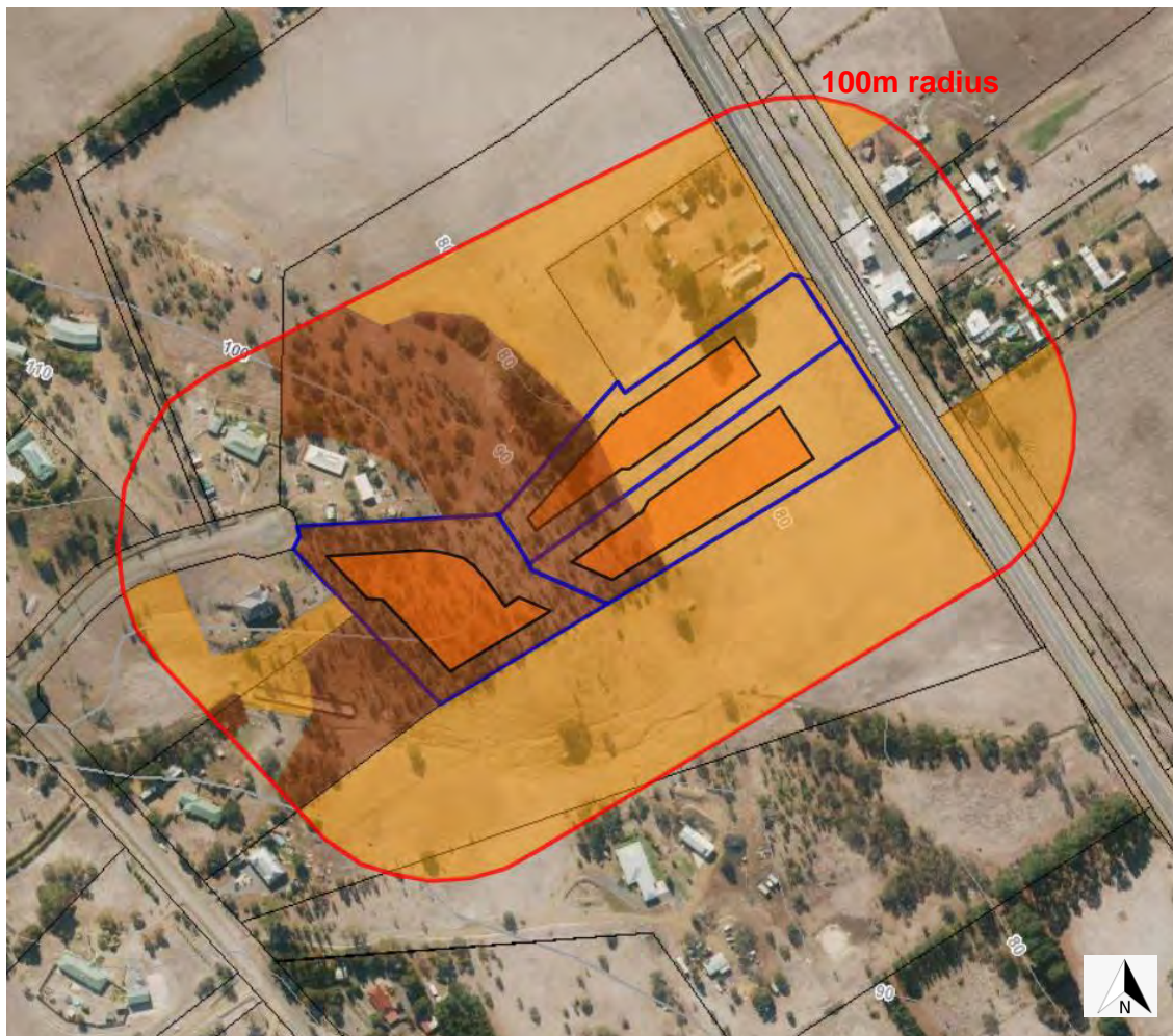
Figure 4: contoured TasVeg4.0 listmap. www.thelist.tas.gov.au Property outline in blue, proposed building areas in orange. Brown shading indicates shrubland bushfire prone vegetation within 100m of proposal and yellow shading grassland.
