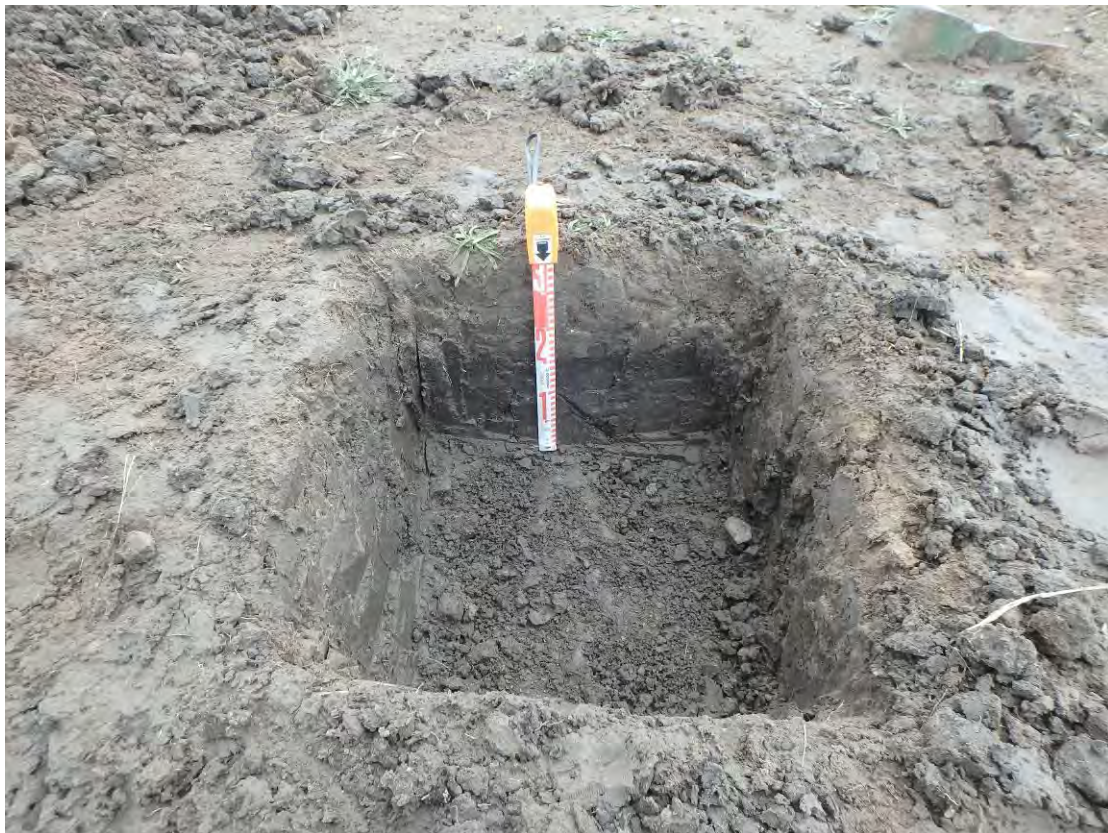
Plate 5: Test pit 6 (east wall) showing the typical soil profile across the test pit zone, with soils comprising homogenous dark brown to grey cracking clays
