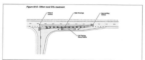
This type of treatment, with a chevron providing separation between the left-turn deceleration lane and the adjacent through lane, was retro-fitted at the Bass Highway / Gilbert Street junction and there have been no further crashes since its implementation.
